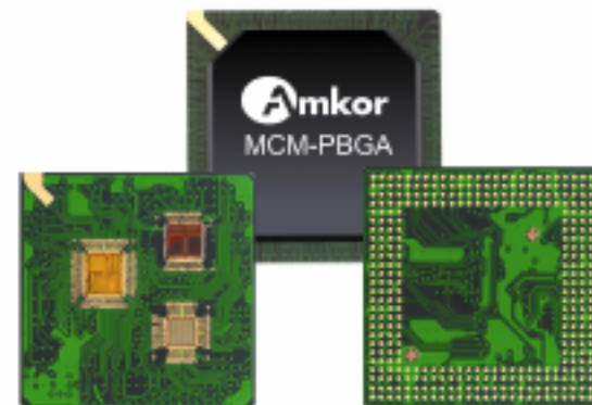
Example of a Multichip BGA with Three Different Dice
